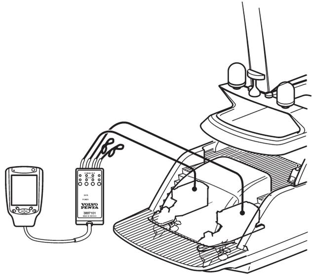
The **switch box (1)** is connected to starboard and port engine diagnosis connection and the VODIA tool is connected to the switch box. The switch box makes it possible to switch between the drive legs during the operation.
