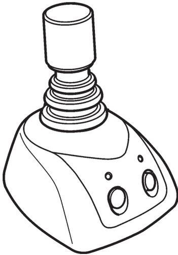
The joystick unit is connected to the steering system (the CAN bus) by the use of Y-split cables, length 2.5 m (8.2 ft). The mounting hole diameter is 52 mm (2.05").
