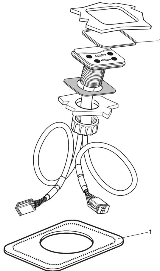
Make a hole for the button panel using the template enclosed with the installation kits. Also refer to the **Templates for controls and panels** chapter .
