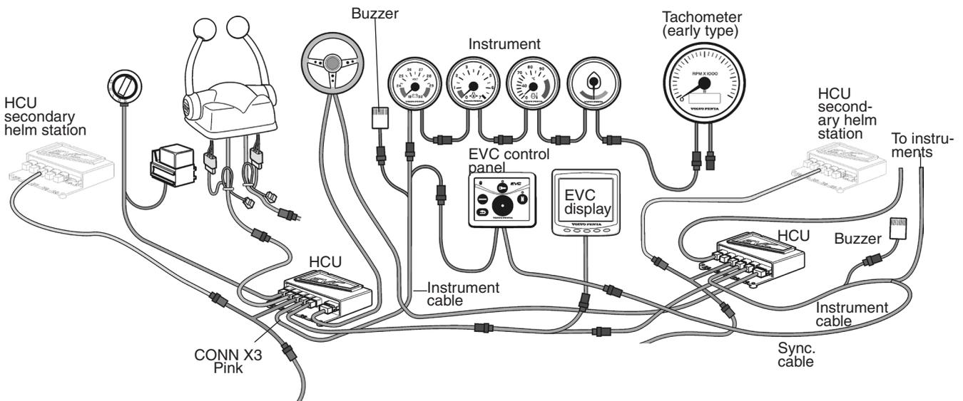
This cable is optional. It is used when an EVC system display is installed and an additional buzzer is required.
