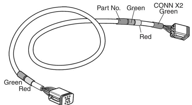
The cable must only be used to connect the PCU to the HCU.
