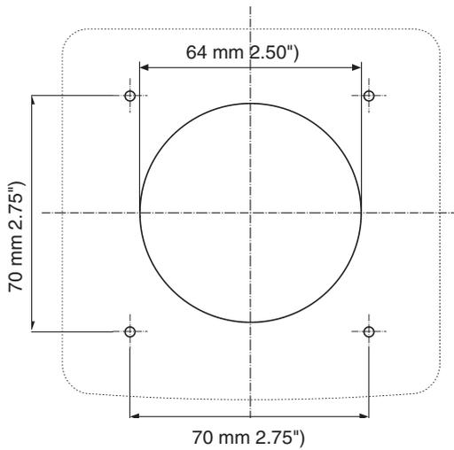
rear side with a diameter of 65 mm (2.56") and drill the four Ø 4.3 mm (0.17") holes for the studs. See the **Templates for controls and panels** chapter .
