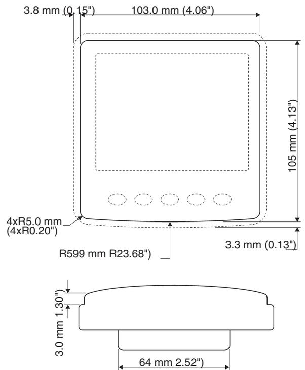
Make a hole for the display using the template enclosed with the installation kits. Use tailor made fittings. Also refer to the **Templates for controls and panels** chapter .
