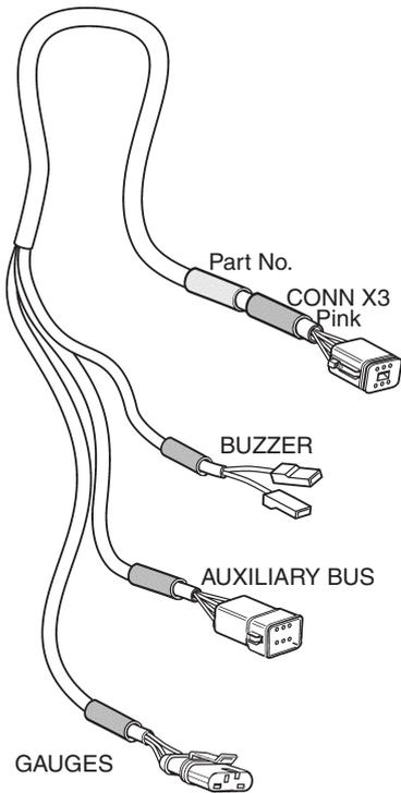
This cable harness is used when an EVC display substitutes a tachometer and/or when you need an additional buzzer. The harness connects the HCU to the instrument bus cable (easy link), the auxiliary bus and the buzzer .
