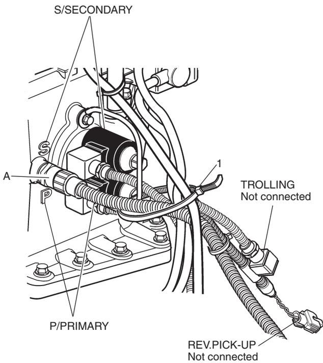
**NOTE!** Check the markings P (PRIMARY) and S (SECONDARY) on the gearbox housing.
