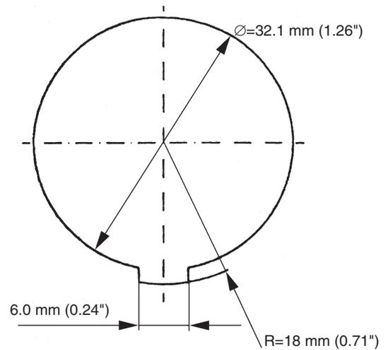
Locate a dry, suitable place for the switch and make a hole according to the drawing.
