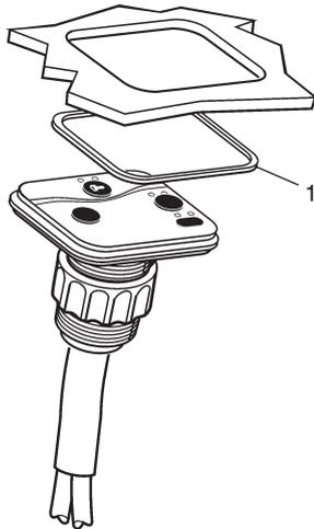
Refer to the **Start/stop panel** section for assembling instructions. Figure shows a panel for twin engine installation.
