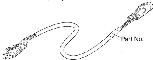
Connection of instrument to instrument when distance exceeds 220 mm (8.6").
