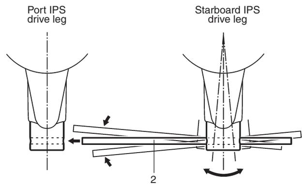
Then move the bar to the starboard cylinder and repeat the steps above until the bar aligns with the port cylinder hole.
