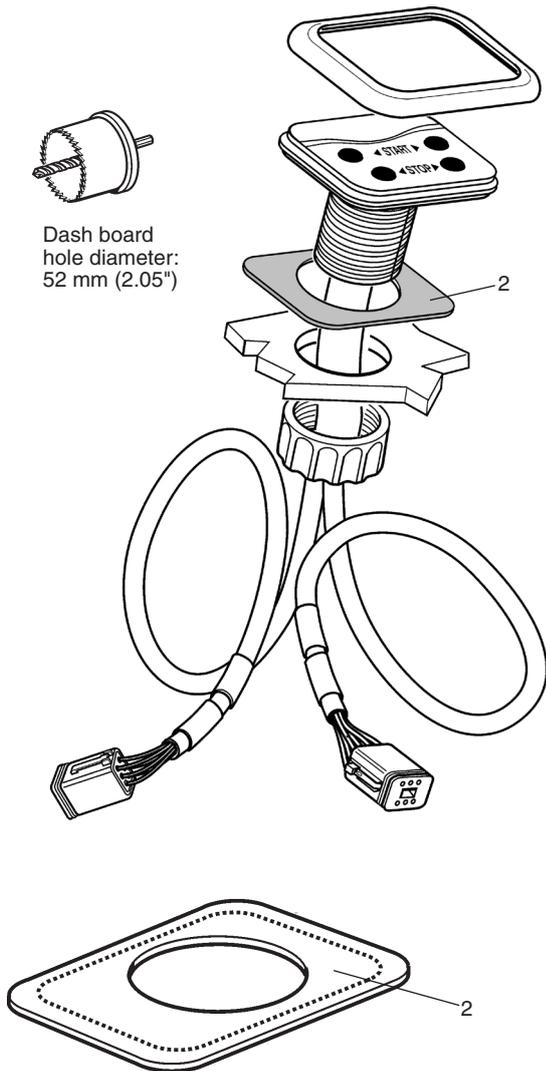
Make a hole for the button panel. The hole must be of diameter 52 mm (2.05").
