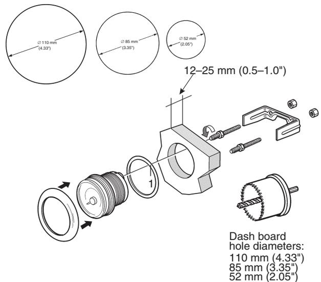
Make a hole, diameter 110 mm (4.33"), 85 mm (3.35") or 52 mm (2.05") depending on type of instrument.
