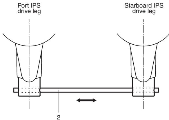
When the bar (2) can easily be moved through the cylinder holes without any resistance the drive legs are in parallel and parallel to the boat keel.
