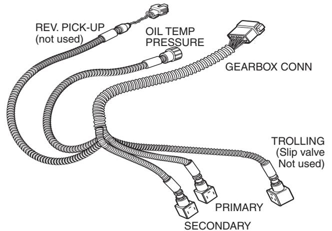
The cable harness has connectors to the gear shift solenoids on the IPS unit, PRIMARY (P) and SECONDARY (S), to the oil temperature and pressure sender on the IPS unit and to the engine – PCU cable. TROLLING and REV. PICK-UP connectors are not used.
