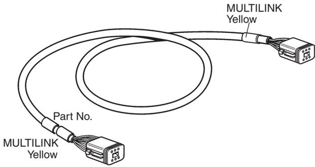
This cable has female/female connectors. It is used to connect the tachometer to the multilink chain.
