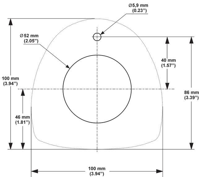
Mark out and make holes for the joystick. A full size template is located in the back of this installation instruction.
