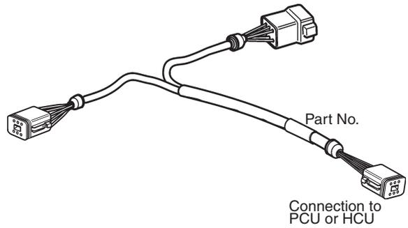
This is avoided by always connecting the longer cable on the Y-connector **directly** to the node (PCU or HCU) without using any extension cable.
