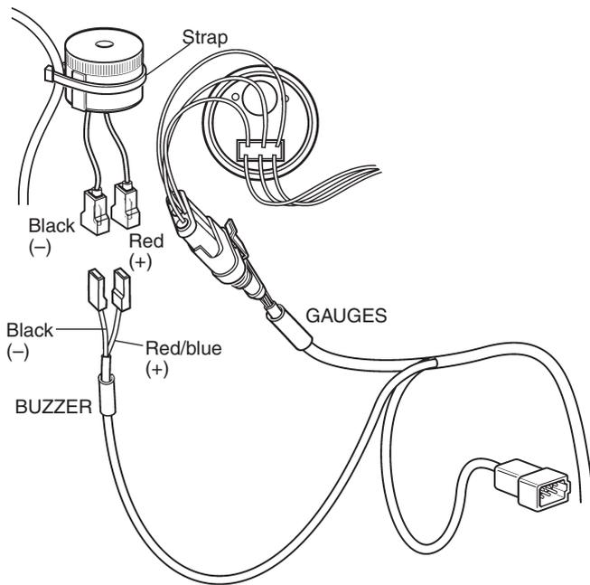
Mount the buzzer under the dash board in an appropriate place by using one or two straps.
