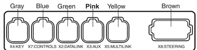
Connect the EVC control panel cable to the connector marked AUXILIARY BUS on the instrument cable harnesses on the HCUs, **red colored** cable coating to port and **green colored** cable coating to starboard engines.
