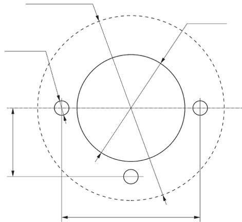
1. Mark out and drill the holes for the bracket (1) using the template. Scale hole templates are included in the **Templates for controls and panels** chapter.
