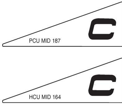
PCUs and HCUs in the EVC-C system have a label fitted on front side with the letter "C" printed on it and with the following marking:
