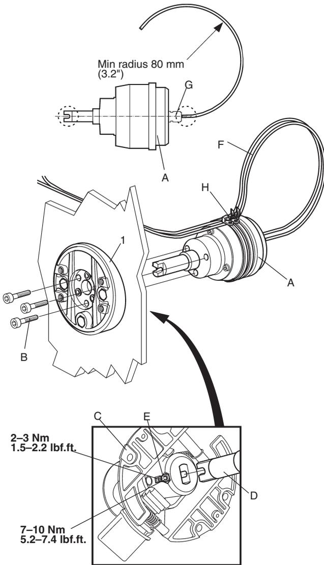
**⚠ IMPORTANT!** Cable connector (G) should be parallel with the spindle, to avoid subjecting it to mechanical side forces. Smallest permissible bending radius for the cables is 80 mm (3.2 "). The cables must not be subjected to strain during or after installation. The cables should be fixed to protect them from sharp bends and vibration. The cables must not be exposed to temperatures exceeding 70°C (158°F). There are no extension cables to the steering cables.
