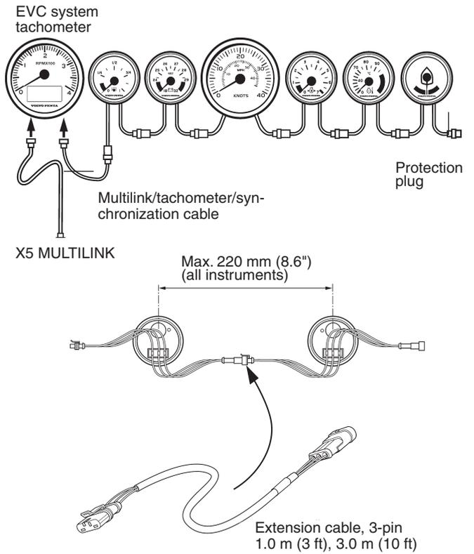
Connect the other instruments to the 3-pin EasyLink connector in the tachometer.
