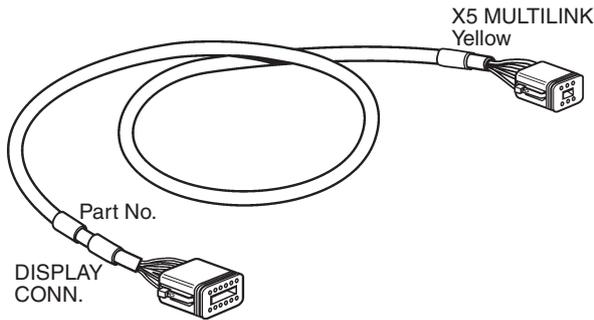
To connect the EVC system display to the multilink cable or the MULTILINK BREAKOUT on the Y-split cable from connection X5 on the HCU.
