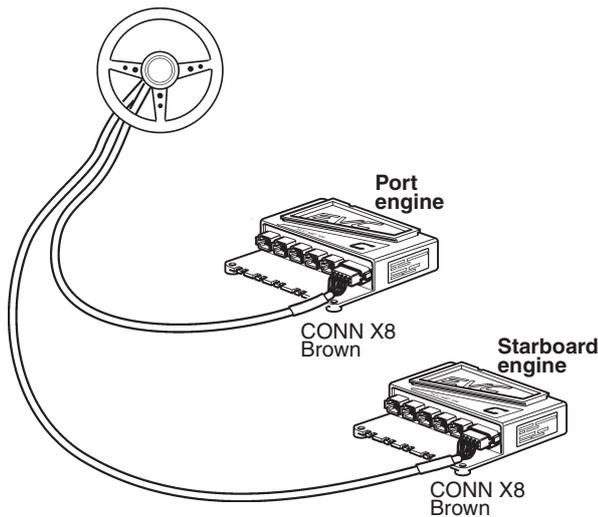
The two steering cables from the steering wheel unit shall be connected to the HCU connection X8: STEERING (brown) starboard and port. It is of no importance which cable is routed to starboard or port HCU.
