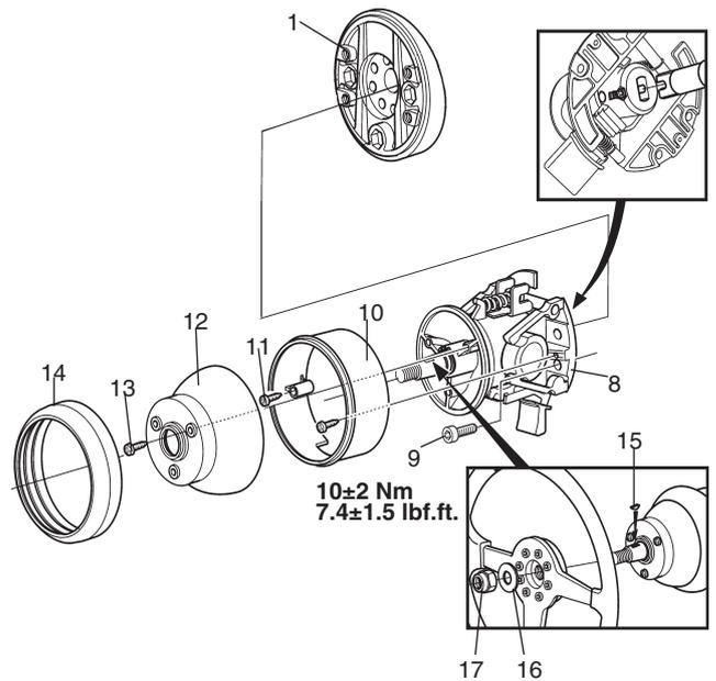
5. Install the steering wheel adjuster (8) on bracket (1) with screw (9) as in illustration.
