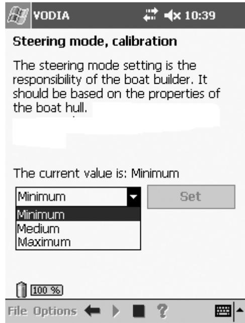
There are three values when setting the steering angles: MINIMUM, MEDIUM and MAXIMUM.
