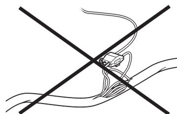
Never cut or modify the Volvo Penta EVC cable harnesses. For extra power supply use the Volvo Penta relay for accessories.
