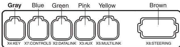
The key switch is connected to the HCU, X4:KEY connection (gray) together with the relay socket for external accessories.
