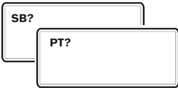
5. One of the tachometer displays will read “PT?” (port engine).
