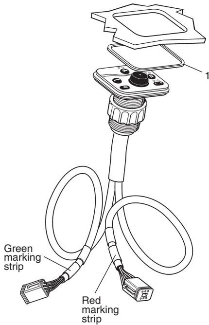
Refer to the **Start/stop panel** section for assembling instructions. Figure shows a panel for twin engine installation.
