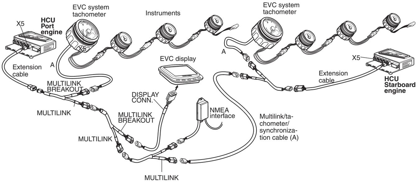
To synchronize the engines a synchronizing cable must be installed between the HCUs for starboard and port engines in a twin installation.
