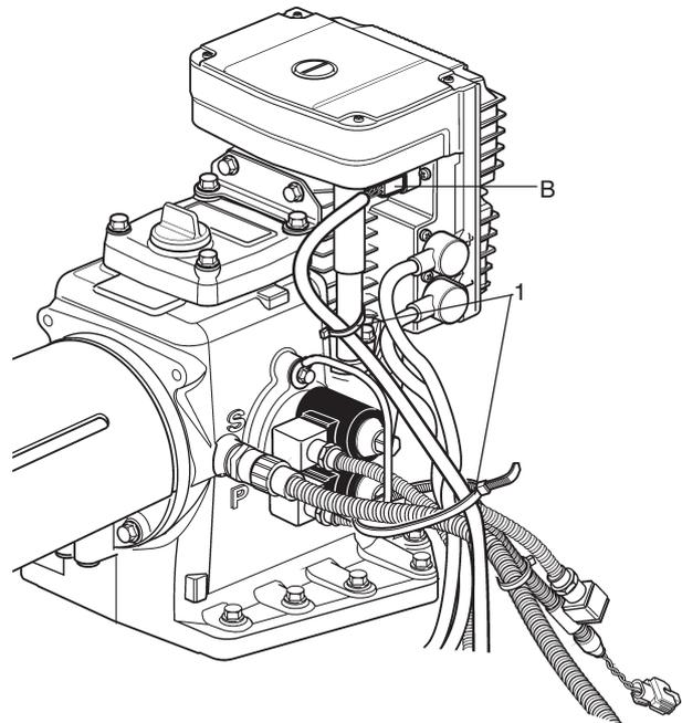
The cable for steering signals from the HCU/PCU is connected to the 6-pin connector (B) on the Servo Unit Steering (SUS).
