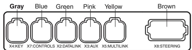
Connect the start/stop control panel cable to the connector marked X4:KEY (gray) on the HCU.
