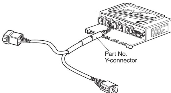
Figure shows the Y-connector fitted to a HCU.
