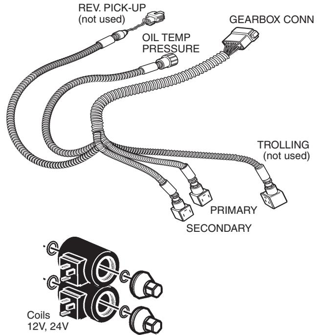
The cable harness connects the gear shift solenoids and the oil temperature and pressure sender on the IPS unit to the EVC system. The harness kit also includes the two connectors/coils to the solenoid valves (12V or 24V), including O-rings.
