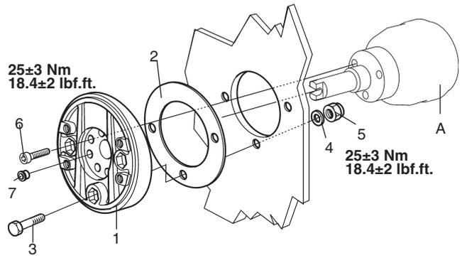
2. Install the gasket (2) and bracket (1) on the instrument panel with three screws (3), washes (4) and nuts (5) as in illustration.
