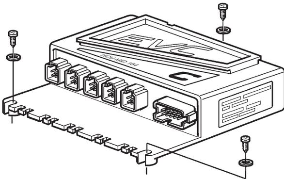
The PCU/HCU nodes shall be fitted with **three** screws.
