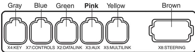
The synchronizing cable is a part of the multilink chain connected to X5: MULTILINK (yellow) on each HCU. See figure above.
