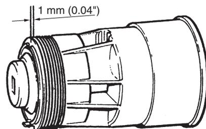
The switch fits to 2 mm (0,08") panel. If the switch is installed in a thicker panel the switch housing can be trimmed by up to 10 mm (0,4"), 1 mm (0,04") between each flute.
