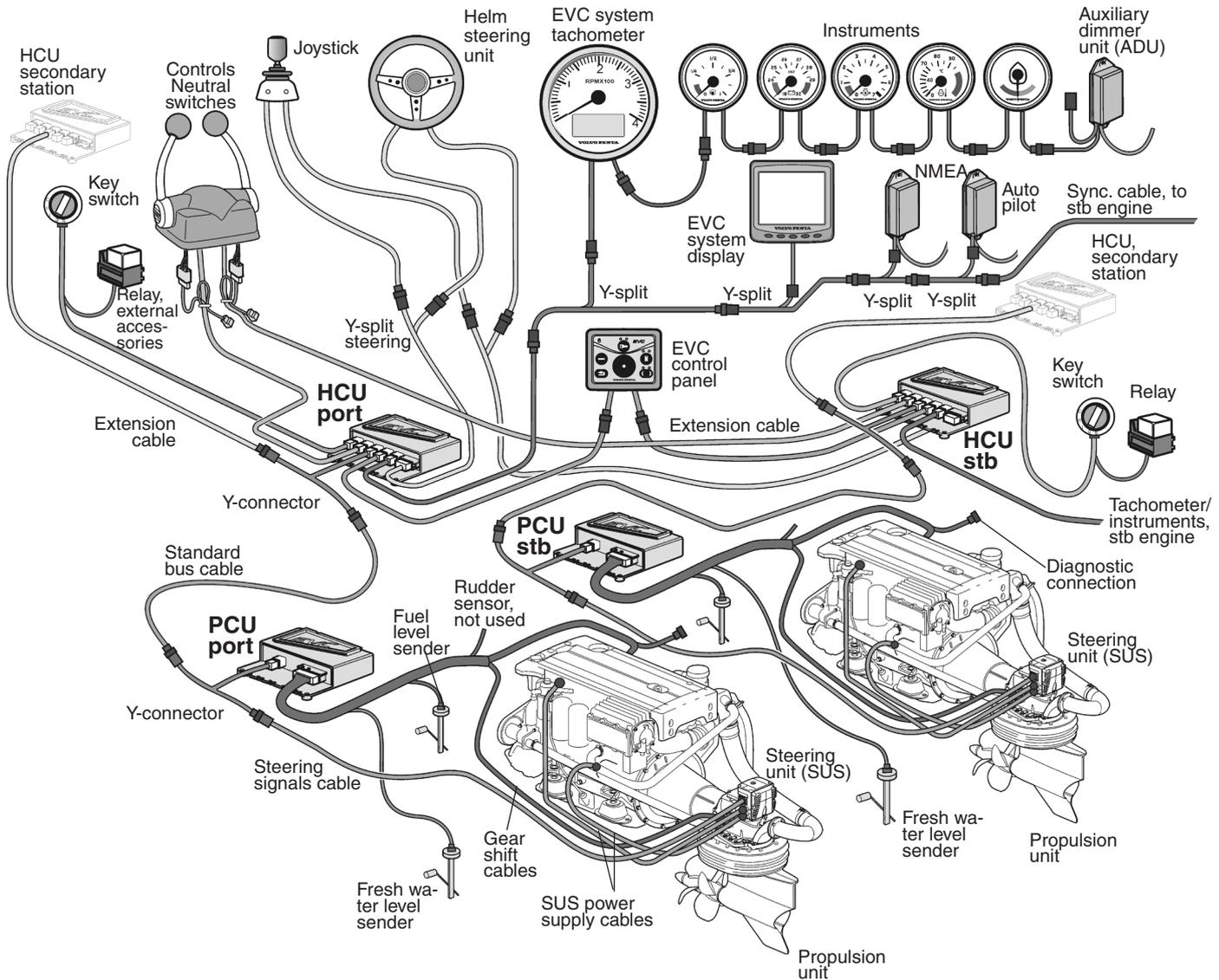
**NOTE!** The nodes are always located close to the components they control. A power train node, the Power train Control Unit (PCU), is located in the engine room. A helm node, the Helm station Control Unit (HCU), is located close to the helm station.
