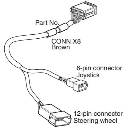
To connect the cables from the helm steering unit and the joystick to the HCU X8:Steering connection.
