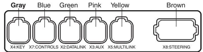
The start/stop panel is connected to the HCU, X4:KEY (gray) or to separate relay cable harness (option).
