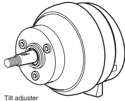
The helm steering unit has a number of position sensors and two cable harnesses, length 2.5 m (8.2 ft). The cables are connected to the HCUs.
