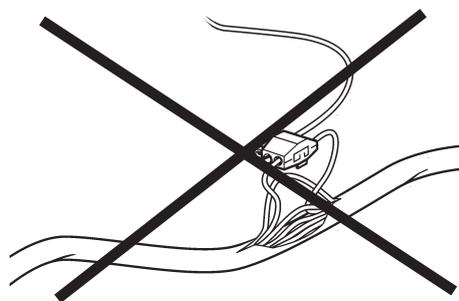
Never cut or modify the Volvo Penta EVC cable harnesses. For extra power supply use the Volvo Penta relay for accessories.
