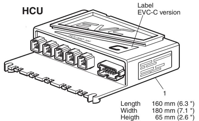
The PCU node is to be located in the engine room. The PCU communicates with the engine and the IPS unit. It also communicates with the helm station control unit HCU, via the standard bus cable.
