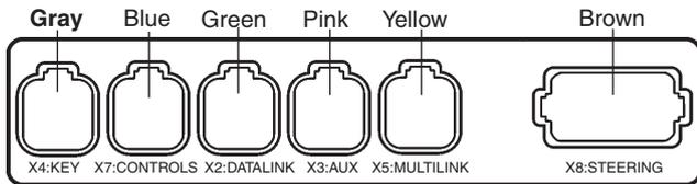
The relay socket is permanently connected to the cable for the key switch. The key switch cable is connected to the HCU, X4:KEY connection (gray).
