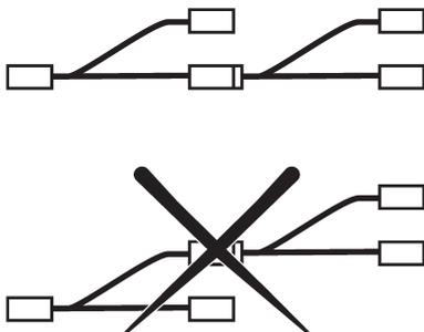
**NOTE!** Do not install a HCU or another Y-split to the MULTILINK BREAKOUT (yellow PVC-coating). If more than one Y-split cable is needed connect them in chain, MULTILINK to MULTILINK.
