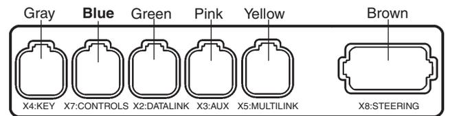
The control cables should be connected to the X7: CONTROLS (blue) connector in the HCU.
