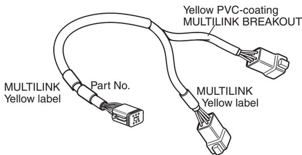
For making branches in the multilink cabling, tachometer-EVC display-sync. connection-NMEA-connection etc.
