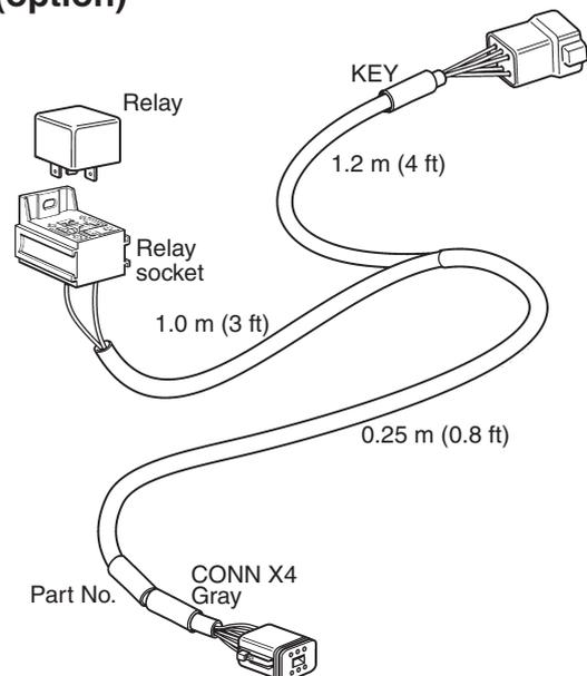
This cable is used in combination with the Start/Stop panel and connects the panel and the relay socket to the HCU. The relay to external accessories shall be mounted on the relay socket.
