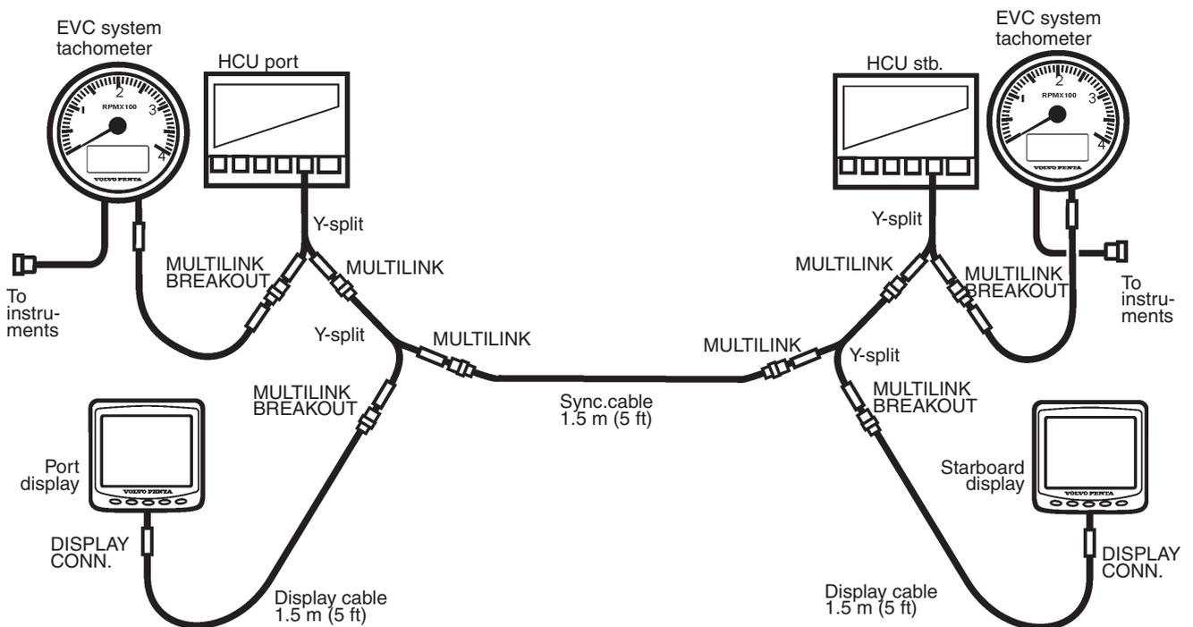
The figure shows a twin installation with two displays, one for each engine. Note that one display can also be used for two engines.
