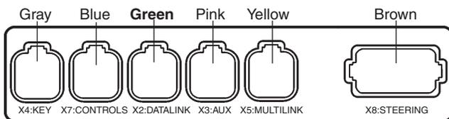
The standard bus cable connects the PCU to the helm station(s), HCU, in the system. It is fitted in the PCU X2:DATALINK connector and the HCU X2:DATALINK connector, that is, cable connector marked CONN X2 (green) shall be fitted in the helm unit.
