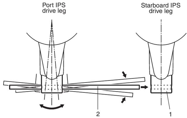
Place the aluminum bar (2) in the port cylinder and use it as an “aligning tool” as shown in the illustration. Carefully position the drive with the bar until the bar aligns with the hole in the starboard cylinder (1).
