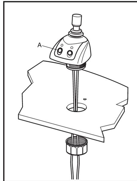
Install the joystick on the instrument panel as in the illustration. The thickness of the instrument panel must not be greater than 25 mm.
