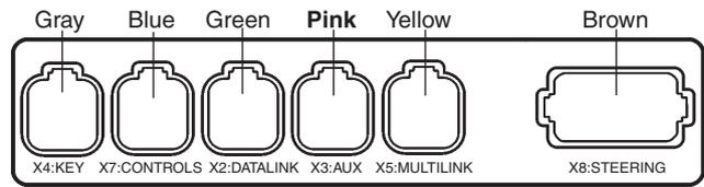
The instrument cable is connected to the HCU X3: AUX connector (pink).
