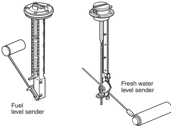
The fuel and water tank levels can be displayed on the EVC display or in separate instruments.
