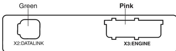
Connect the cable from the engine, marked CONN X3, to connector X3:ENGINE (pink).
