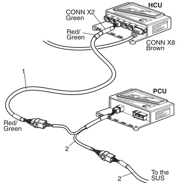
Steering signals are sent via the EVC-bus cable (1) to the Servo Unit Steering (SUS). An Y-connection (2) is used to lead the steering signals past the PCU.
