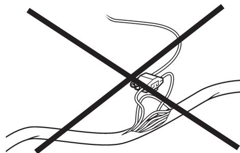
**⚠ IMPORTANT!** Never cut or modify the Volvo Penta EVC cable harnesses. For extra power supply use the Volvo Penta relay for accessories. Refer to the **Relay for external accessories** section.
