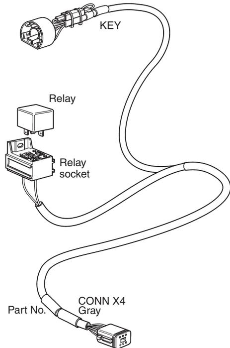
Connects the key switch to the HCU. The relay to external accessories, if used, should be connected to the relay socket included in the cable. Relay has to be ordered separately.
