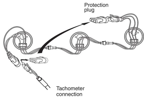
**⚠ IMPORTANT!** Always plug the open end of the instrument cable to prevent corrosion. Use the plug attached to the cable harness.
