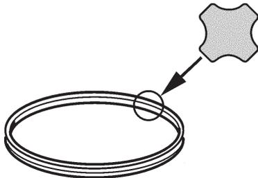
If the instruments should be flush mounted into the instrument panel, a gasket must be fitted to prevent water from entering behind the panel.
