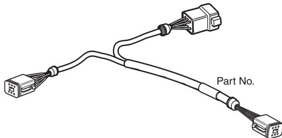
**! IMPORTANT!** The Y-connector must always be connected directly to the PCU (X2) or the HCU (X2) without using any extension cables.
