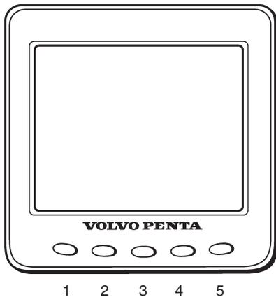
Volvo Penta display EVC system (EVC system display) is an instrument which displays operating information about the engine and allows you to communicate with the engine's electrical system.
