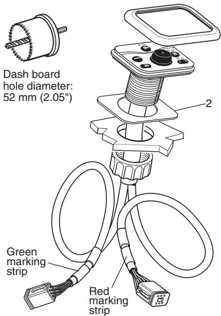
Refer to the **Start/stop panel** section for assembling instructions. Figure shows a panel for twin engine installation.
