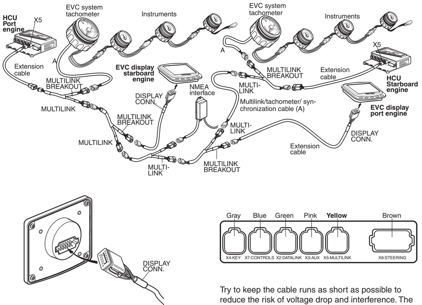
Figure shows a twin engine installation with Y-split cable and synchronization cable.
