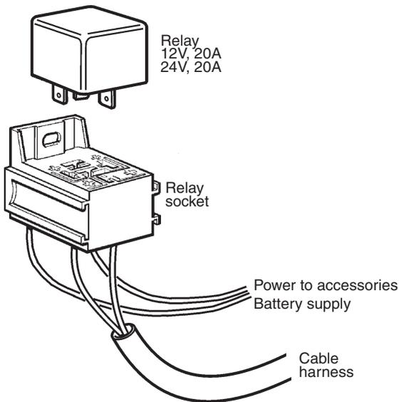
The relay controls the power supply to external accessories. The relay position (open or closed) and the power supply depend on the key switch position. The relay is normally open and there is no power when key switch is in the OFF position.
