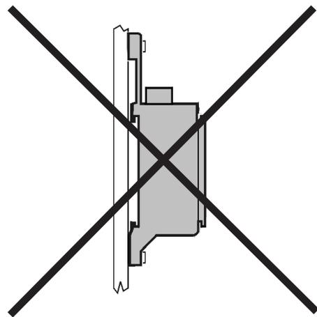
**⚠ IMPORTANT!** Never mount the PCU and HCU units with the connectors pointing upwards.
