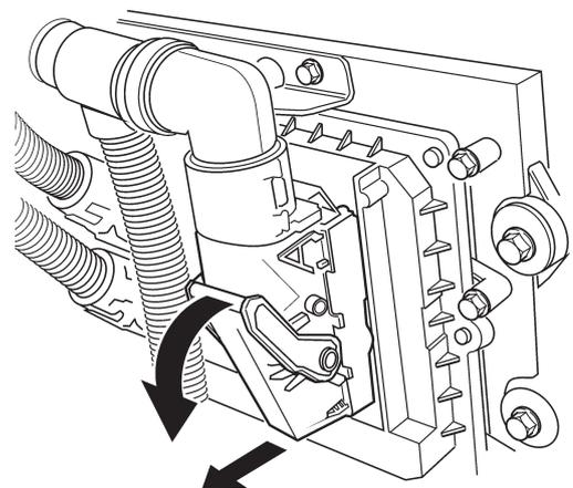
Press the lock tab down and pull the connector out. Refit the connector to the engine control unit after disconnecting the welding equipment.
