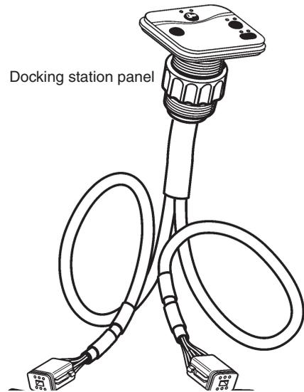
A docking station panel is required to start/stop the engines from a docking station.
