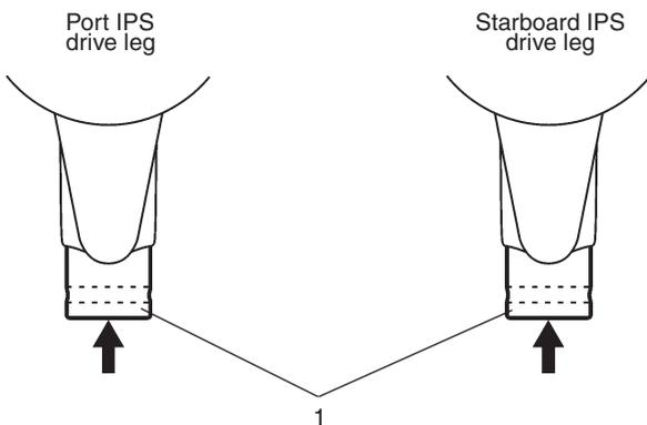
When calibrating, push the plastic cylinders (1) into the exhaust outlets on the drive legs.
