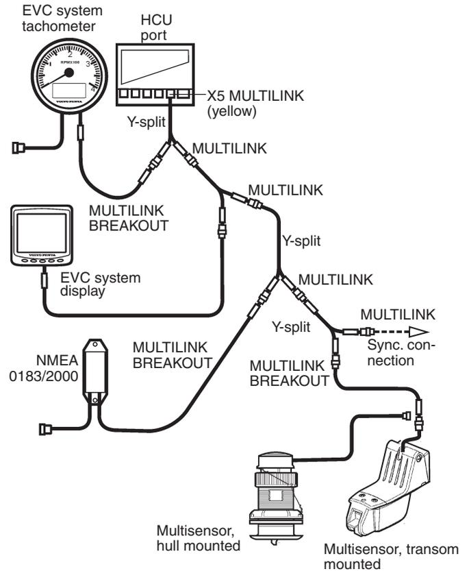
Multisensors are connected to the X5 MULTILINK connector, directly or via the Y-split, MULTILINK BREAKOUT cable (yellow PVC coating).
