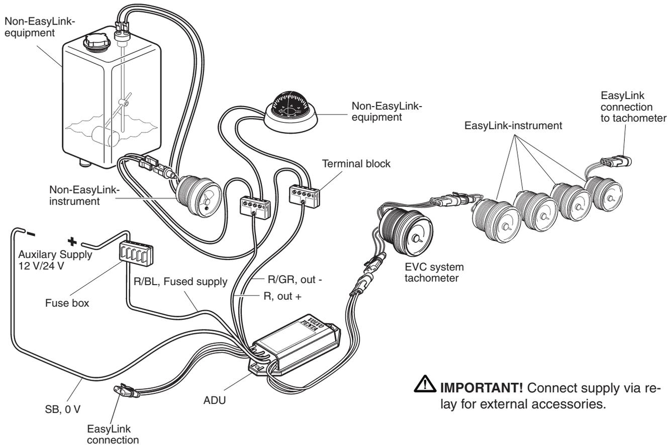
**⚠ IMPORTANT!** Connect supply via relay for external accessories.
