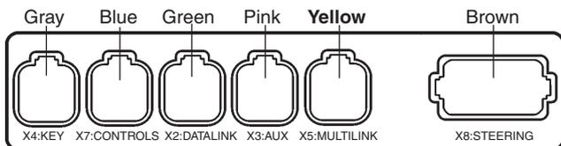
Connect the EVC system tachometer to the HCU connection X5 (yellow). Connect directly to X5 using a multilink/synchronization cable.
