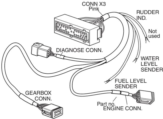
The cable connects the PCU to the engine, IPS unit (gear box), fuel level sender (black PVC-coating) and fresh water sender (blue PVC-coating).
