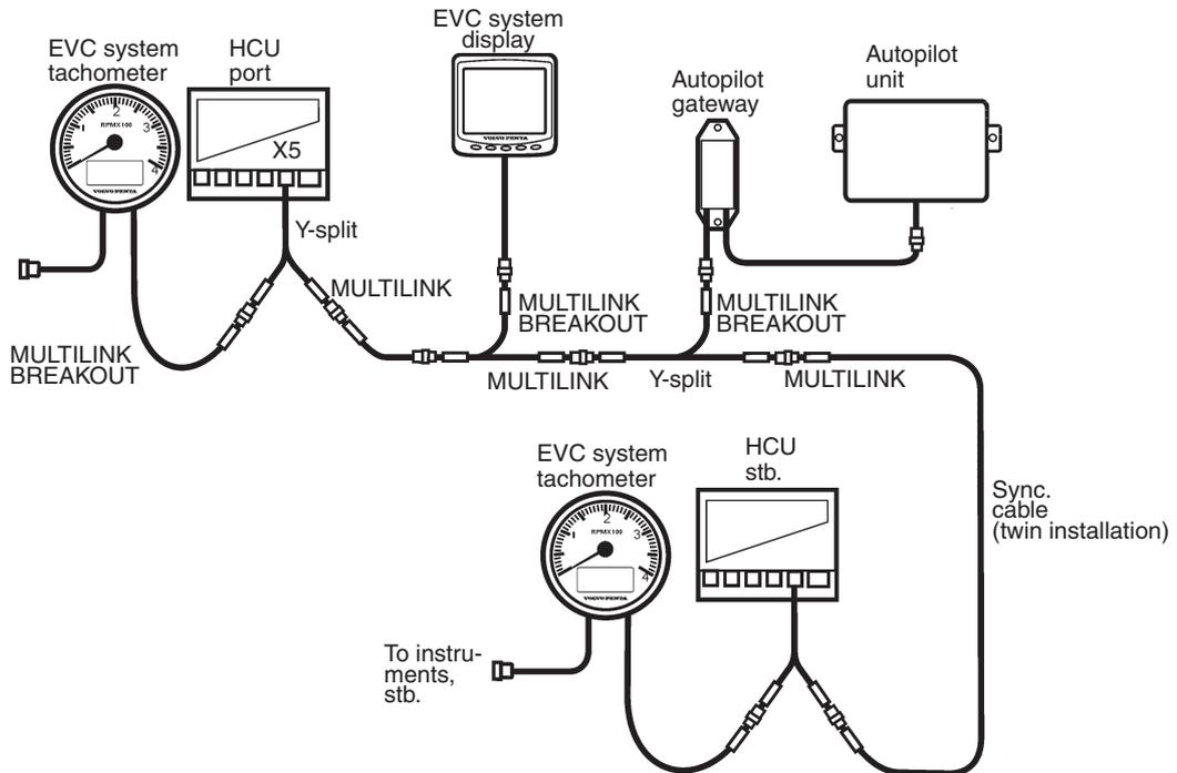
Connect the connector marked MULTILINK BREAK-OUT on the Y-split cable to the Autopilot gateway connector (6-pin).
