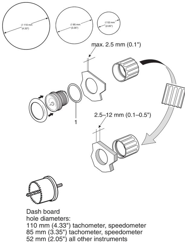
**NOTE!** An attaching nut is used when dash board thickness is up to 12 mm (0.5"). If dash board thickness is greater than 12 mm (0.5"), please refer to **Instrument with attaching clamp** on the next page.
