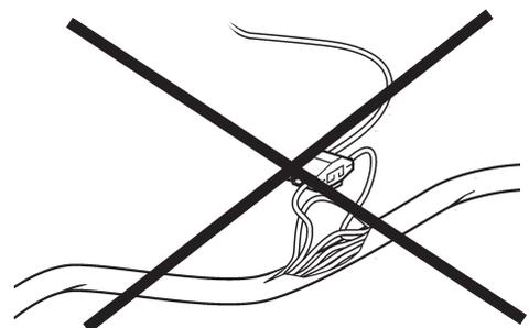
**⚠ IMPORTANT!** Never cut or modify the Volvo Penta EVC cable harnesses. For extra power supply use the Volvo Penta relay for accessories. Refer to the **Relay for external accessories** section.
