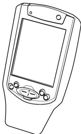
The VODIA diagnostic tool can be used to adjust EVC-parameters. This is done with the "**Parameter programming**" tool in the "**Service and maintenance**" menu.
