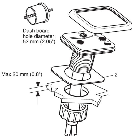
Refer to the **Start/stop panel** section for assembling instructions. Figure shows a panel for twin engine installation.
