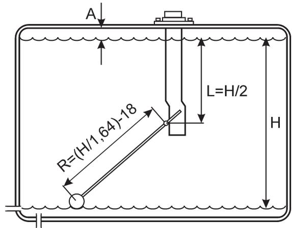
**NOTE!** Never use the fuel level sender as a freshwater sender. Corrosion problems can occur.
