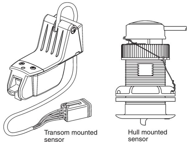
The multisensor is available in two designs, for transom mounting and for hull mounting. The multisensor submits data of boat speed, water depth and water temperature. Data can be shown in the EVC display. The speed data is also available in an instrument (speedometer).
