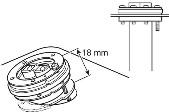
Lower the sensor with float and the ring with tapped holes down into the tank. The rubber seal must be outside the tank. Align the sensor so that the float has free movement inside the tank. Tighten the long screw so that the seals and the ring with the tapped holes come into place. Install the remaining screws and tighten all of them simultaneously.
