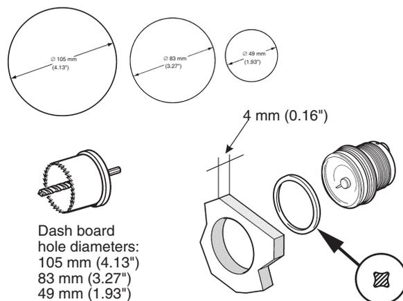
Insert depth should be 4 mm (0.16").
