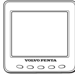
The Volvo Penta EVC system display is an on-board instrument for indication of engine operating values, boat speed and other data. The display consists of a self-contained, computerised unit for fixed installation on a dash board. A Liquid Crystal Display (LCD) screen is used for data presentation.
